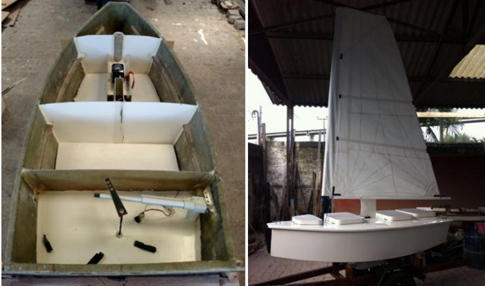
Figure 4. ASV: construction steps of the N-Boat II.
