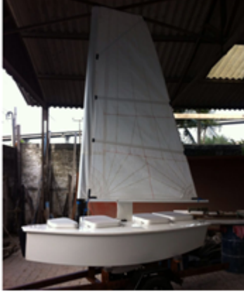
Fig. 1. N-Boat II Robot measuring 2.5 meters in length
