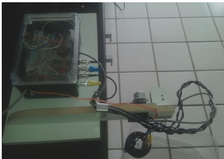
**Figure 5.** Physical system prototype, in the bottom it can be seen a piece of wood with a spool (attached to a servomotor) where it runs the thread that put the sensors in and out of the water; the electronic circuit prototyped in a board can be seen in the top left box (will be seen in detail in Figure 6); the sensors are (waterproof) coupled at the end of the braided cables seen in the right bottom.
